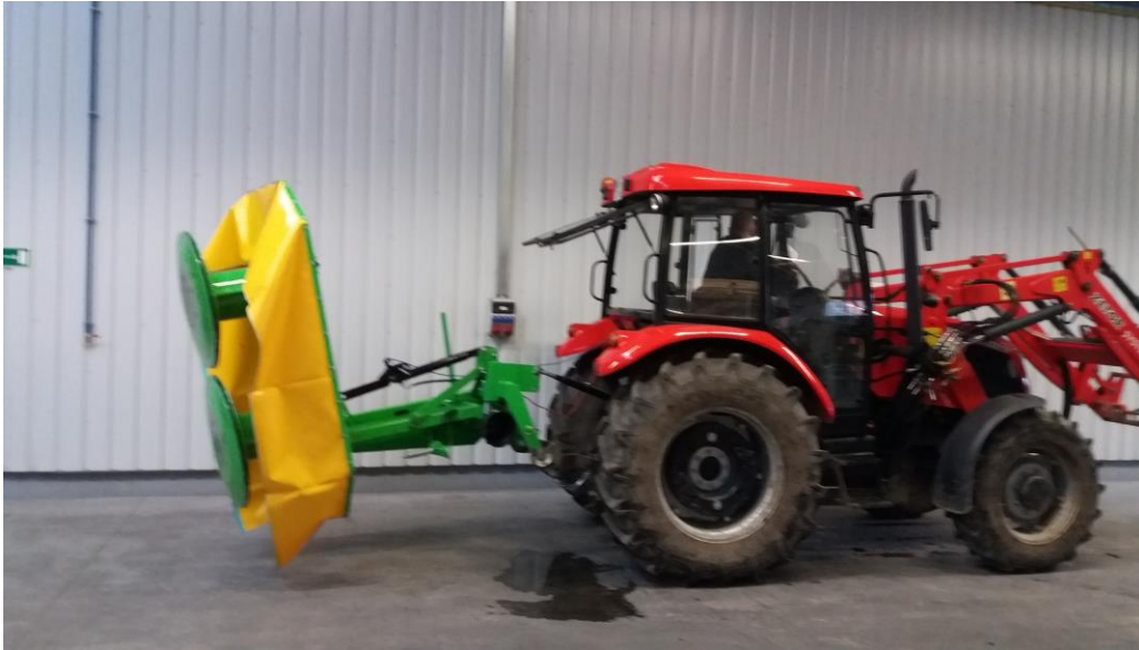
Figure 9 Proper transport position for 1.85m and 1.65m mowers in the hydraulic cylinder version
