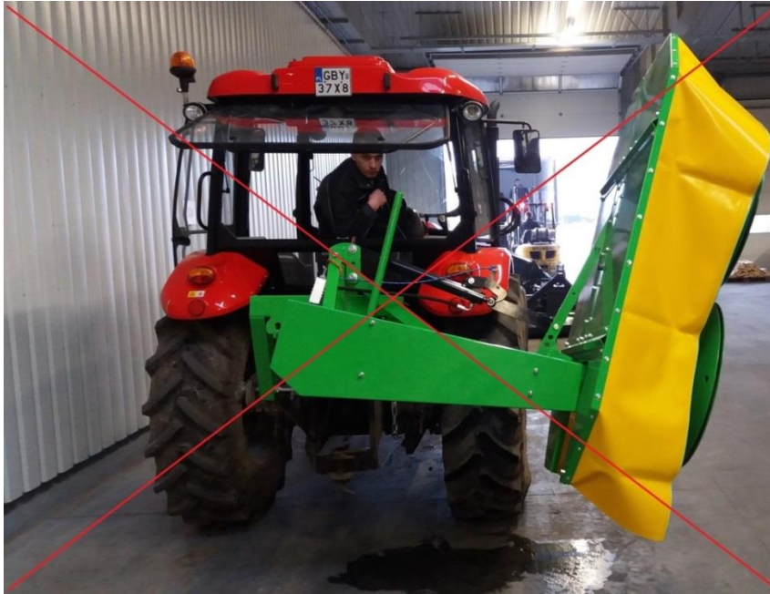
Figure 12 Incorrect transport position for 1.85m and 1.65m mowers in the hydraulic cylinder version (the transport width above the permissible value.)
